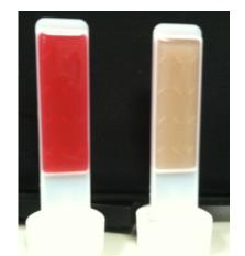
**Figure 3.** Representative dip-slide with double agar sides free of microbial contamination. This dip-slide was used to test the LoxaSperse dispersion for up to 24 h of environmental exposure.
