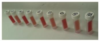
**Figure 2.** Dip-slide tubes used for testing LoxaSperse dispersion at 1, 2, 3, 4, 5, 6, 7, 8 and 24 h after the powder contents were mixed with sterile water.
